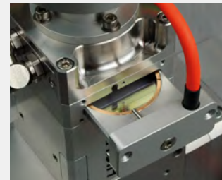
Cover slide for additional protection of collimation
